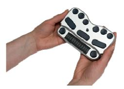
The BraillePens can act as fully-functioning Windows keyboards, with all the capabilities of a standard PC keyboard. BraillePen Write software, which enables this, is supplied with every BraillePen and BraillePen 12. You can also configure special keymaps, so that they can be used for 6-key entry into specialist programs such as Braille Translation software.
