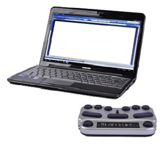
The BraillePens support Bluetooth connections with the main types of Bluetooth providers. These may be built in to a device, or they may be a USB-based add-on for a PC or netbook.
